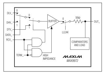
Figure 2. Multiplexer and Driver Channel
