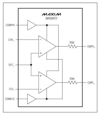
Figure 3. Complementary 50Ω Comparator Outputs
