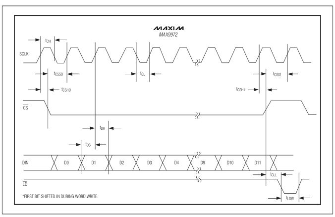
Figure 5. Serial-Interface Timing
